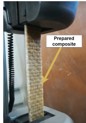
Figure 6. Tensile test of the composite.
