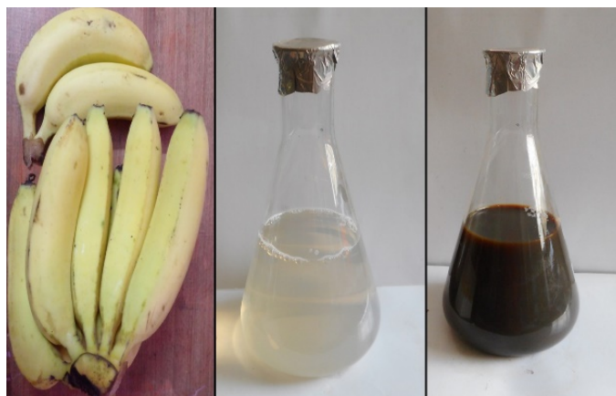
Figure 1. Colour change from pale yellow to brown indicates the synthesis of silver nanoparticles
