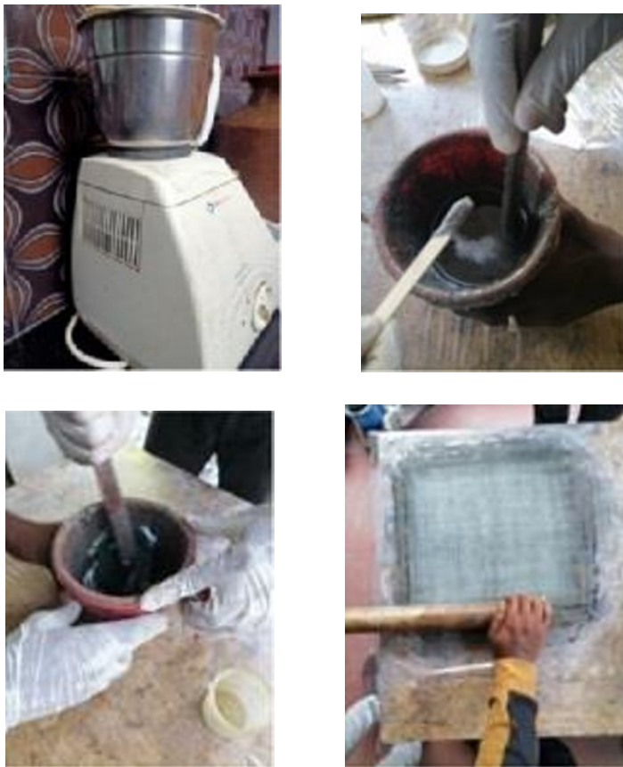
Fig. 1. Mobile display powdered in Mixer and mixed in the epoxy resin and made up using hand layup method
