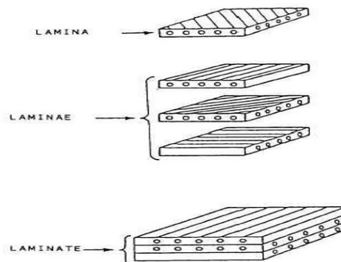
**Figure 2.** Lamina arrangements
