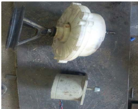
Figure-2. Planetary gear setup and synchronous dynamo.
