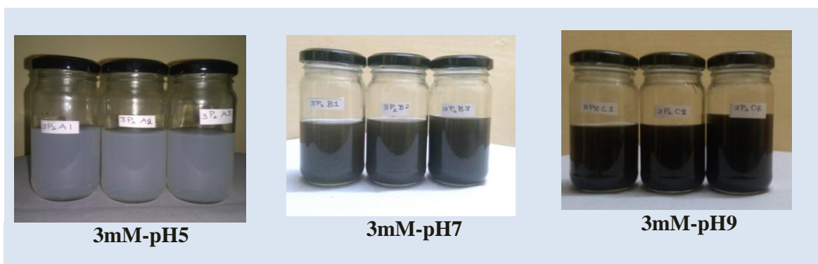
Fig 2: Optimization of Florisynthesis of AgNPs at different pH, concentration of silver nitrate and floral extract of Cordia sebastena
