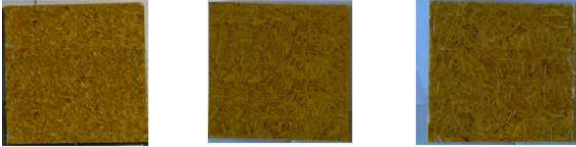
Fig 1. Composite specimens (BF+GF) with 10, 15 & 20mm fiber length and 15% volume fraction.
