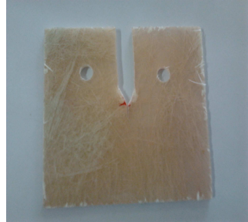
Fig 2 Glass fiber composite of (100×100×3) mm, each provides 13, 17, 20% of fiber respectively and having 10mm fiber length.
