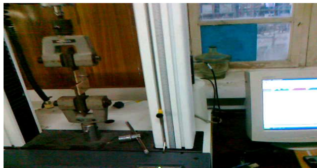
Fig.5 Test Specimen fitted in Instron 4204 Universal Testing Machine
