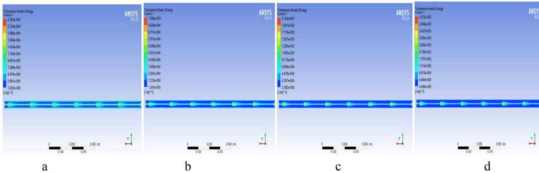
Fig. 10. Turbulence KE Contour with  $\text{Al}_2\text{O}_3$ -Water nanofluid at Re (a) 2000 (b) 5000 (c) 7000 and (d) 10,000.
