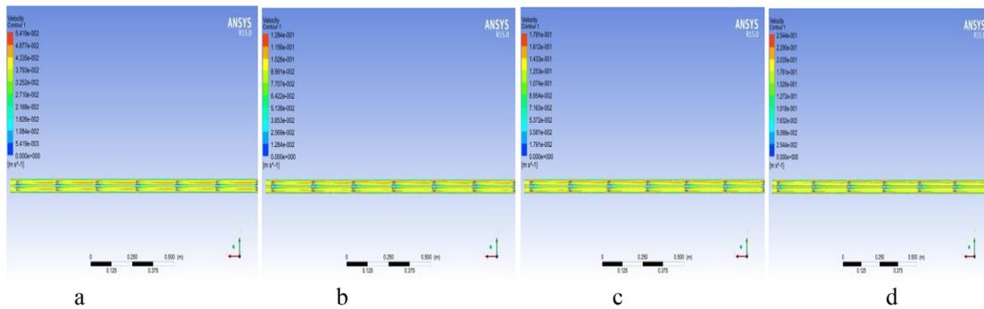
Fig. 11. Turbulence Velocity Contour with  $\text{Al}_2\text{O}_3$ -Water nanofluid at Re (a) 2000 (b) 5000 (c) 7000 and (d) 10,000.
