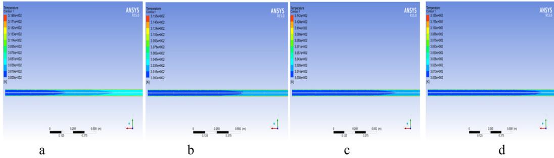
Fig. 13. Temperature Contour with CuO-Water nanofluid at Re (a) 2000 (b) 5000 (c) 7000 and (d) 10,000.
