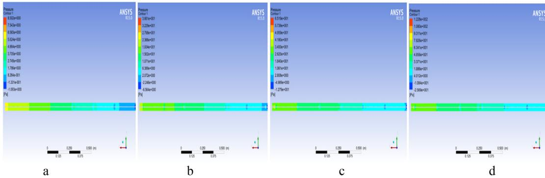
Fig. 8. Pressure Contour with Al<sub>2</sub>O<sub>3</sub>-Water nanofluid at Re (a) 2000 (b) 5000 (c) 7000 and (d) 10,000.
