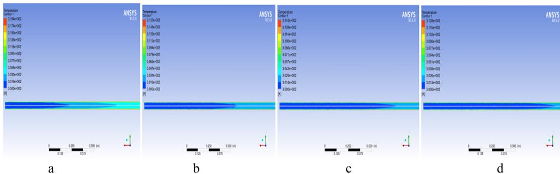
Fig. 9. Temperature Contour with Al<sub>2</sub>O<sub>3</sub>-Water nanofluid at Re (a) 2000 (b) 5000 (c) 7000 and (d) 10,000.
