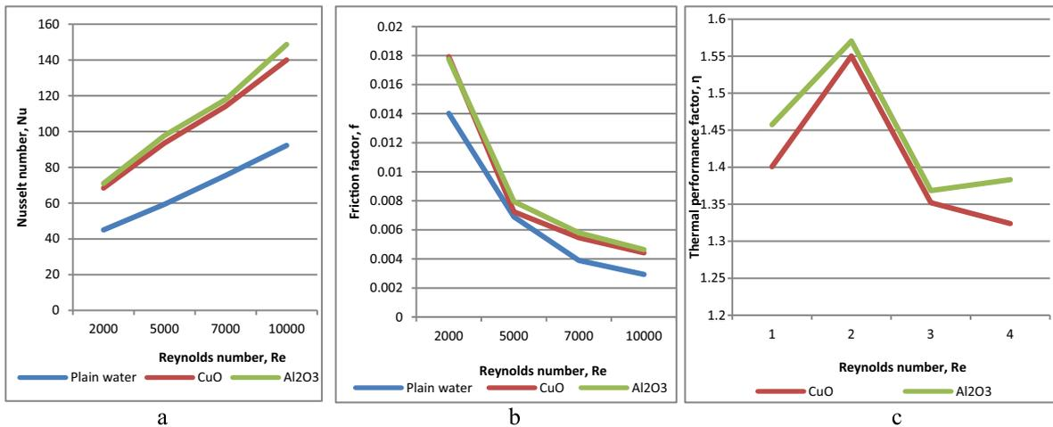
Fig. 16. (a) Thermal performance (b) friction factor and (c) Thermal Performance factor.
