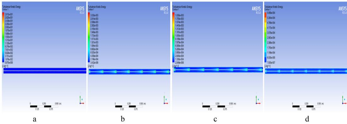
Fig. 6. Turbulence kinetic Energy with plain water at Re of (a) 2000 (b) 5000 (c) 7000 (d) 10,000.
