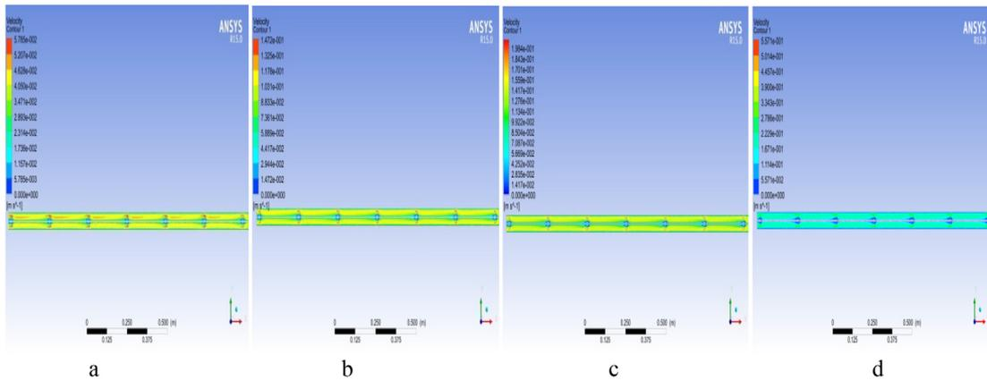
Fig. 7. Velocity contour with plain water at Re of (a) 2000 (b) 5000 (c) 7000 (d) 10,000.
