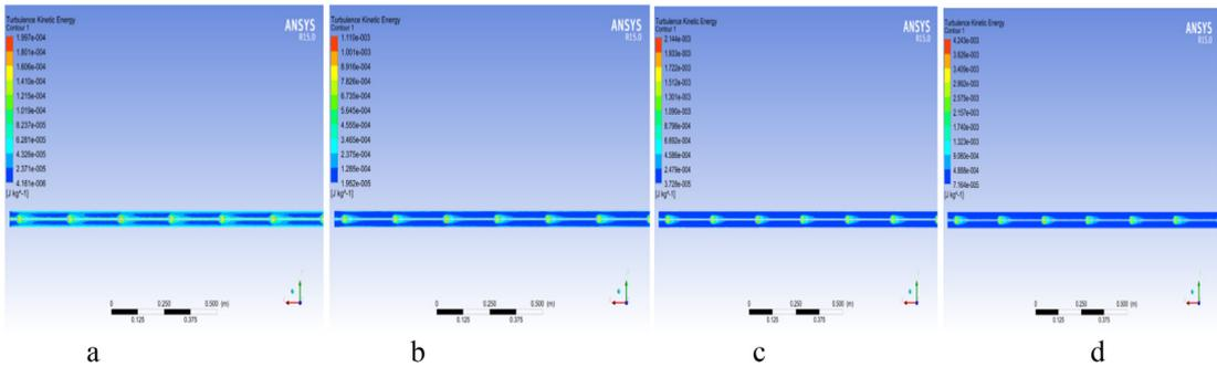
Fig. 14. Turbulence KE Contour with CuO-Water nanofluid at Re (a) 2000 (b) 5000 (c) 7000 and (d) 10,000.
