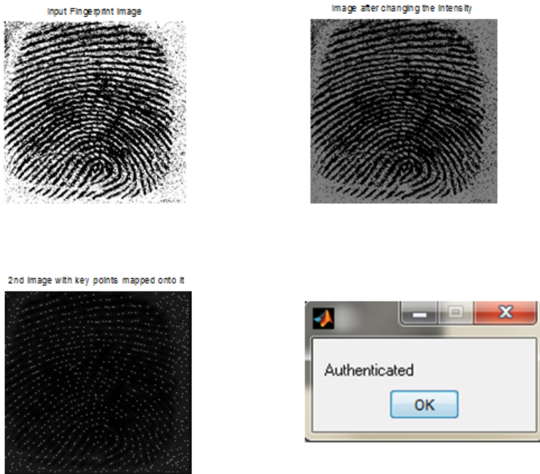
Figure 21 Simulated result of Fingerprint authentication (see online version for colours)
