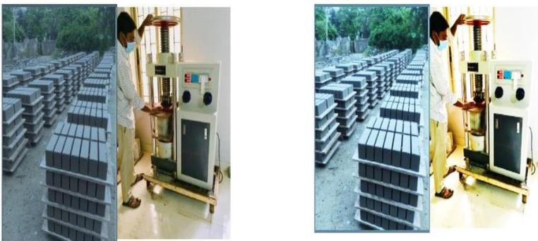
**Fig.3.** Compressive strength test by UTM machine of PMSWA Solid Block.
