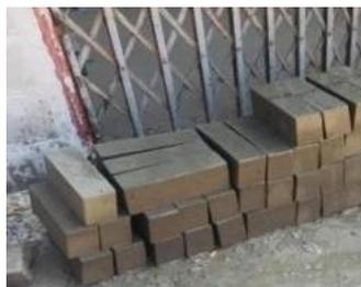
**Fig.2.** Water Curing of PMSWA block.
