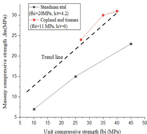
Fig.5. Effect of unit strength on the compressive strength of un-grouted PMSWA block masonry.
