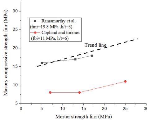
**Fig.6.** Effect of mortar strength on the compressive strength of ungrouted PMSWA block masonry.
