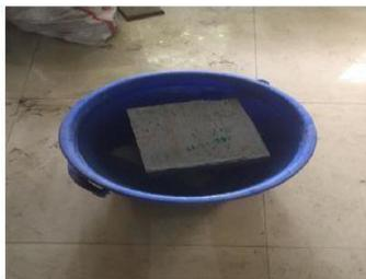
Fig.4. Water absorption of PMSWA Block.
