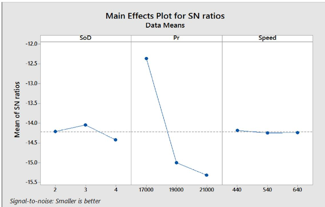
Fig. 7. S/N ratio graph for Ra.
