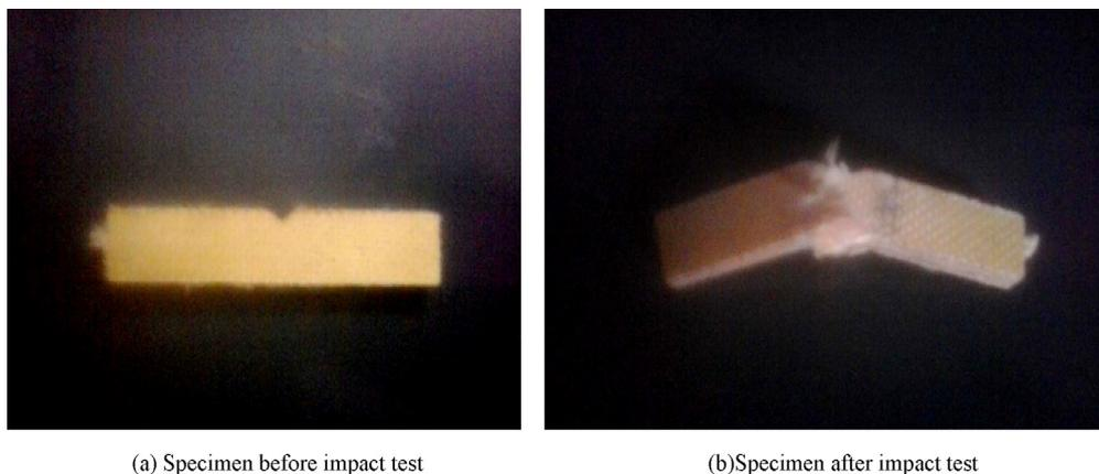
(a) Specimen before impact test
