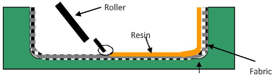
Fig. 3. Hand lay-up process.
