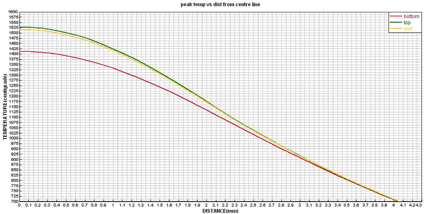
Fig. 4.2. temperature distance curve from weld centre line on top surface and plane 2 mm from top surface at time 20th sec.
