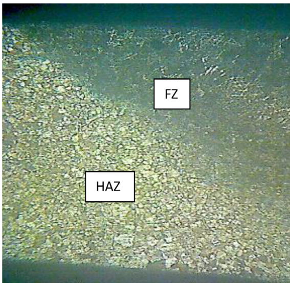
Fig. 4.10. Microstructures 200X coarse grains at HAZ.
