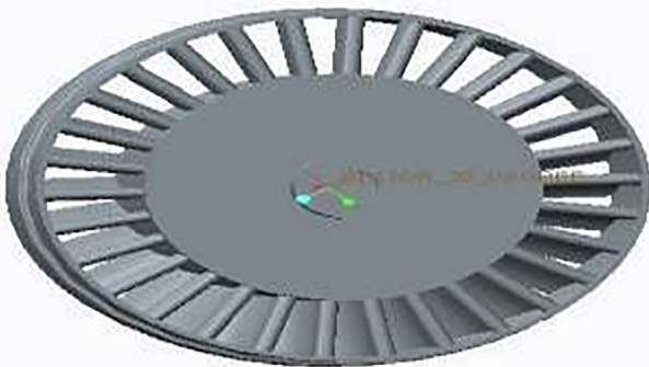
Fig. 3. Stator with blade angle 25°.
