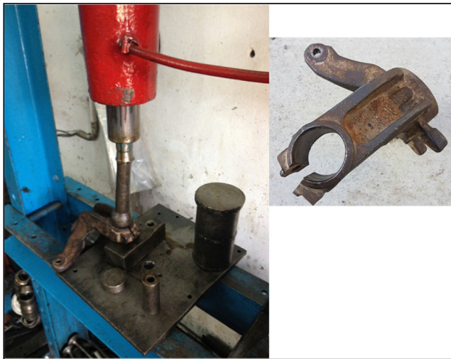
Fig. 9. Photograph of Knuckle Joint Failure.
