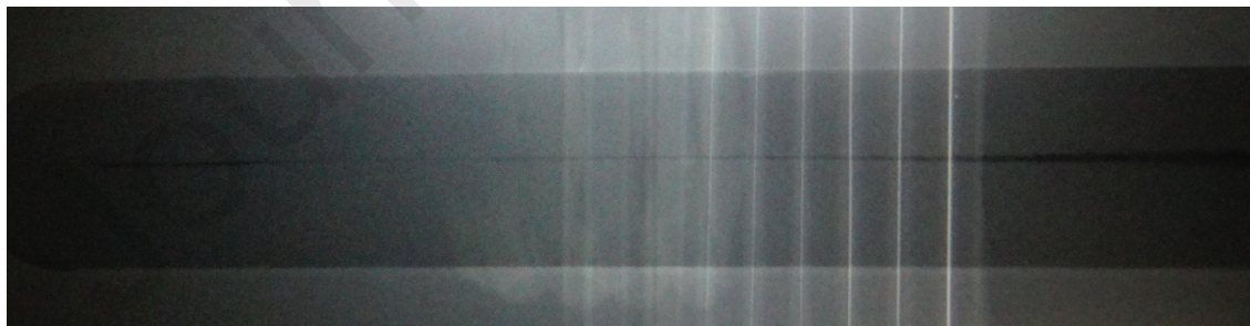
Fig X-ray Radiographic image of weld joint produced at best process parameter from Taguchi method.
