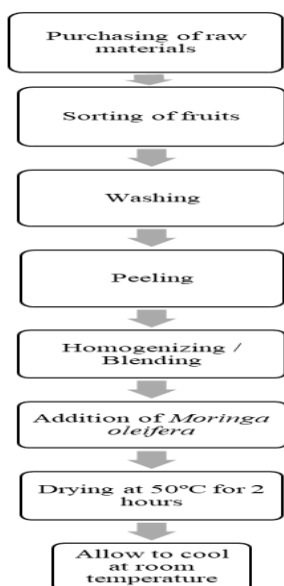
Fig. 1: Flowchart for preparation of fruit leather
