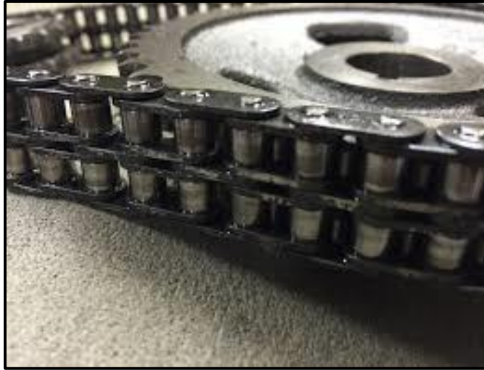
FIGURE 4. Assemble of double chain strip
