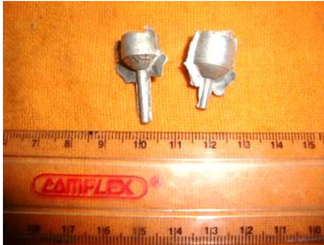
FIGURE 2. Extruded Billet by Channel Die
