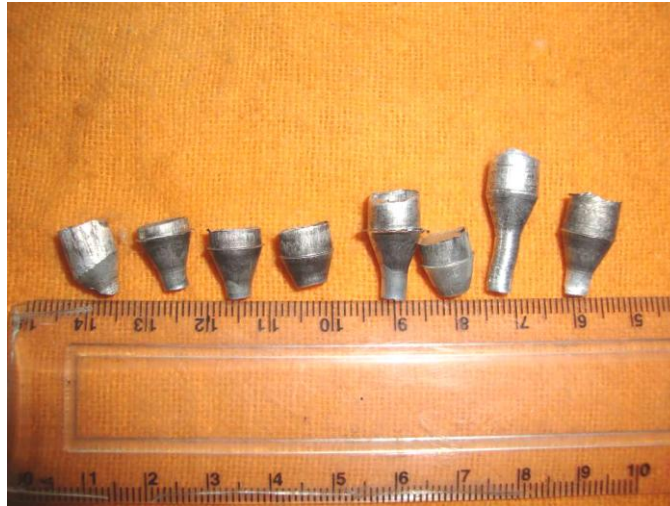
FIGURE 6. Extruded Billet by Three Components Circular Die Set
