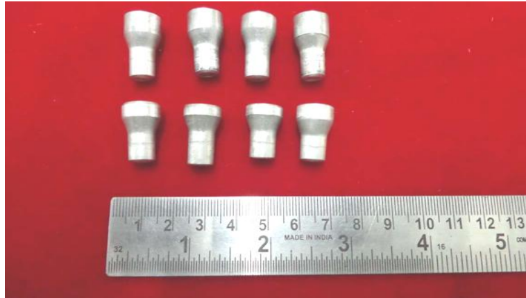
FIGURE 8. Extruded billet by two components circular die set
