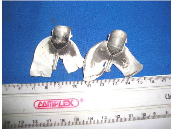
FIGURE 4. Extruded billet by rectangular die
