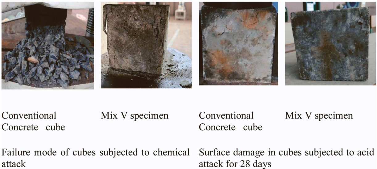
Fig. 8. Failure mode and surface damage in cubes subjected to chemical attack.
