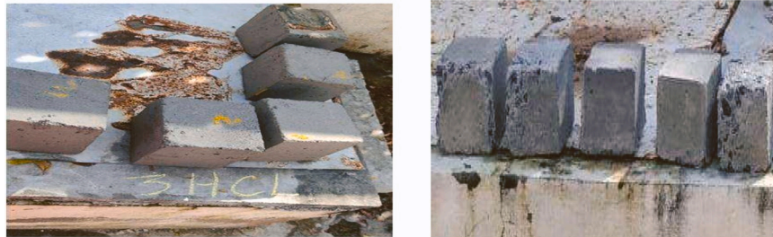
Fig. 5. Cubes immersed in hydrochloric acid and sulphuric acid for 28 days.
