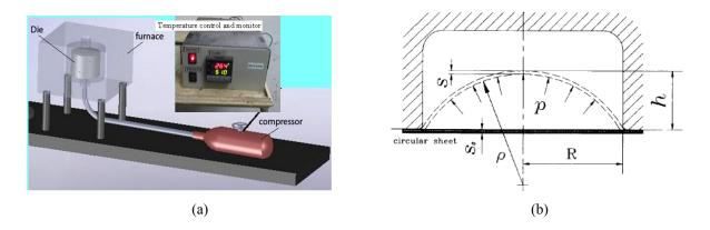
FIGURE 3. (a) Schematic View of superplastic Forming (b) Schematic diagram of superplastic forming process
