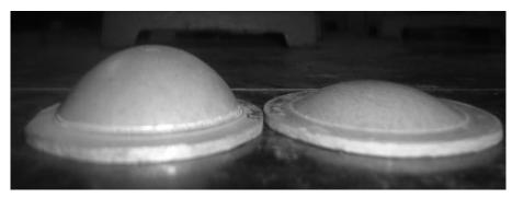
FIGURE 4. Formed at 5 bar 580° C and At 3 bar 580°C
