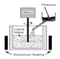
FIGURE 1.Schematic Diagram of Stir Casting
