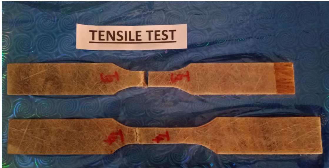
FIGURE 1. Specimen before and after tensile test
