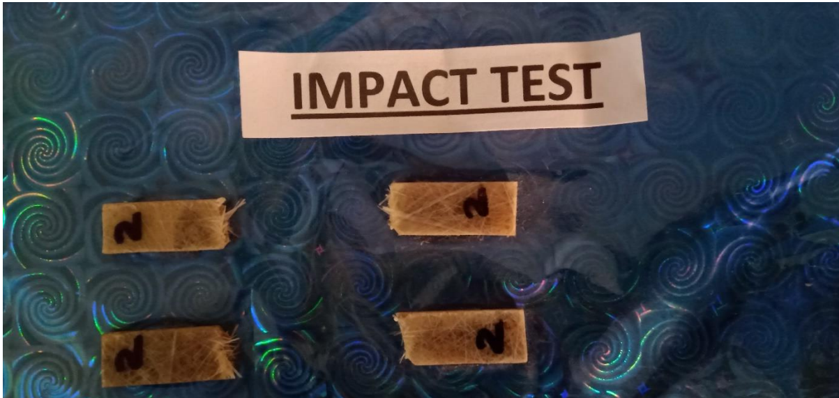
FIGURE 5. Specimen before impact test with V-notch
