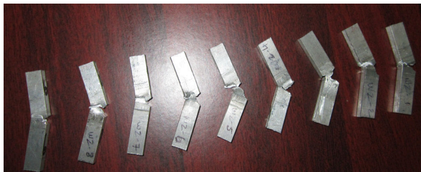
Figure 5. Impact test specimen after fracture
