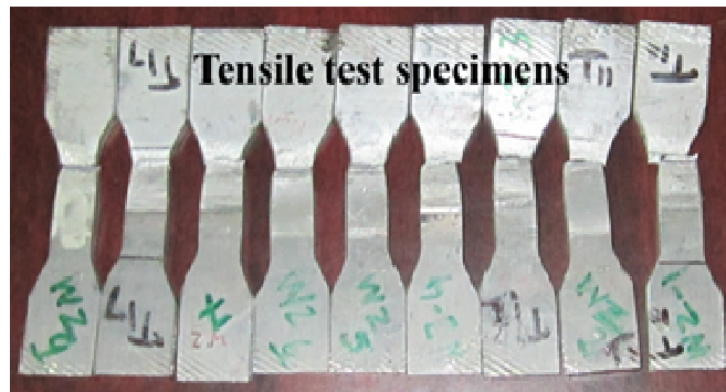
Figure 3. Tensile test specimen after fracture
