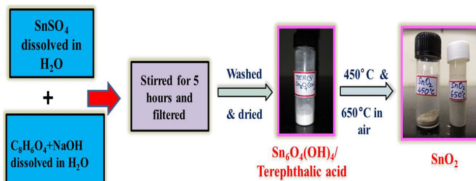
Fig. 1 Diagrammatic representation of the synthesis process for the SnO 2 nanoparticles
