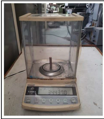
Fig. 8. Electronic weighing machine (Courtesy: National Institute of Technical Teachers' Training and Research, Chandigarh, India).
