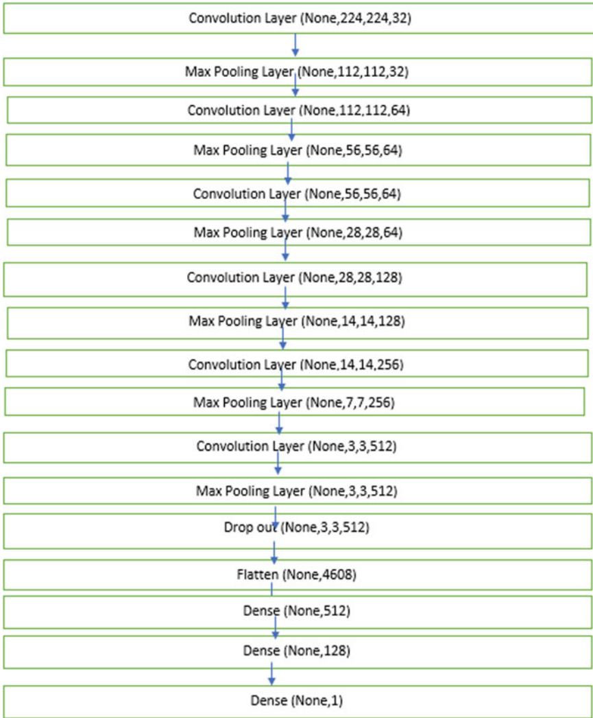
Fig. 7 CNN architecture model for hard exudates detection
