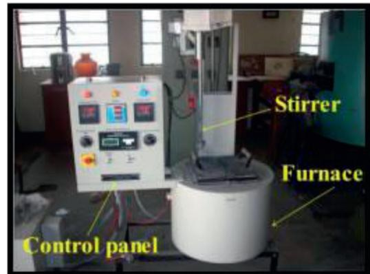
FIGURE 2: Bottom pouring stir casting.
