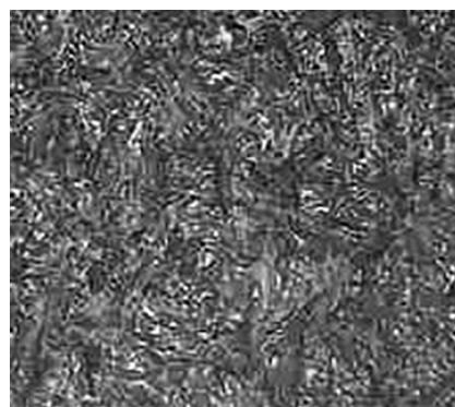
Fig. 4.1. Microstructure at 250 °C Tempering temperature.
