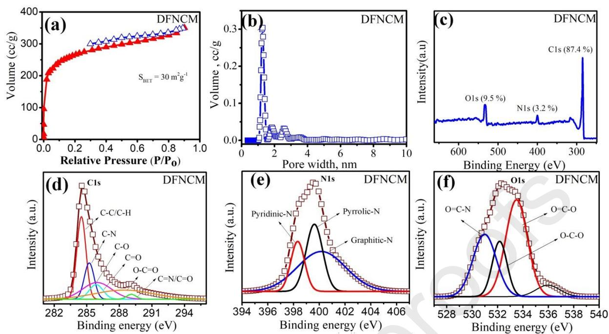
**Figure 2 (a) BET (b) PSD and (c-f) XPS studies (C1s, N1s, O1s) of DFNCM**
