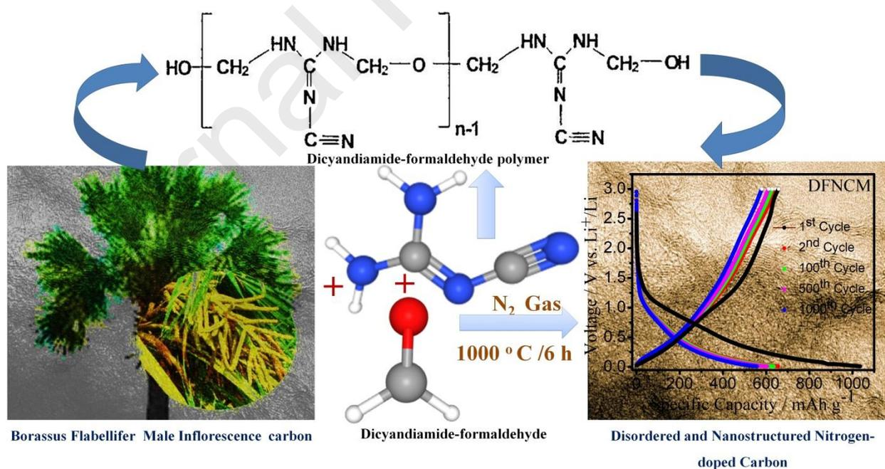
**Schematic illustration of Dicyandiamide-Formaldehyde Condensate Assisted Synthesis of disordered and hierarchically nanostructured nitrogen-doped carbon material.**
