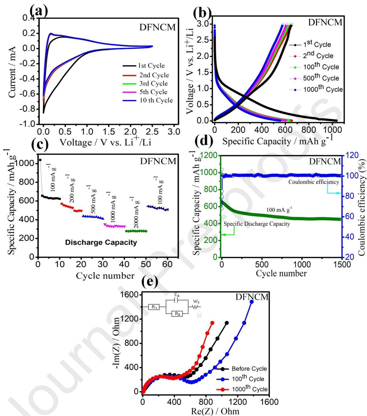
**Figure 3** (a) Cyclic voltammety studies, (b) GCD studies at different cycles, (c) GCD at different current density, (d) Cycling studies at 100  $\text{mA g}^{-1}$ , (e) EIS at before and after cycles.
