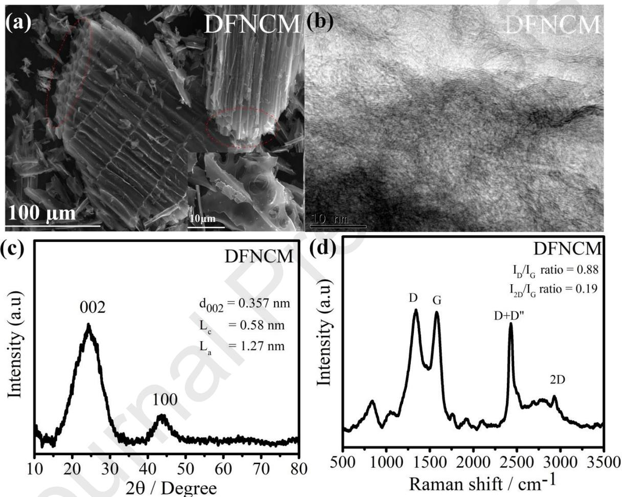
Figure 1 (a) FESEM, (b) HRTEM (c) XRD pattern and (d) Raman spectrum of DFNCM and included Synthesis of Dicyandiamide-formaldehyde polymer- Reaction mechanism
