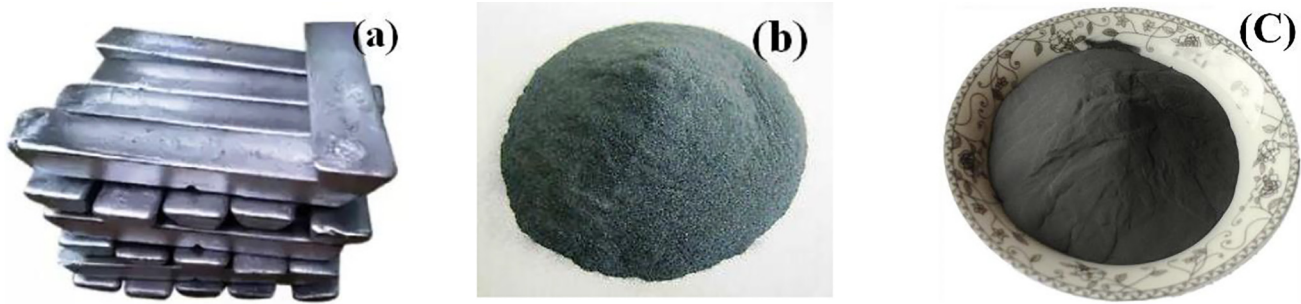
Fig. 1. Hybrid Aluminum matrix composite Materials elements (a) LM 16 alloy ingots, (b) Sic Particles and (c) Nickel-coated Graphite.
