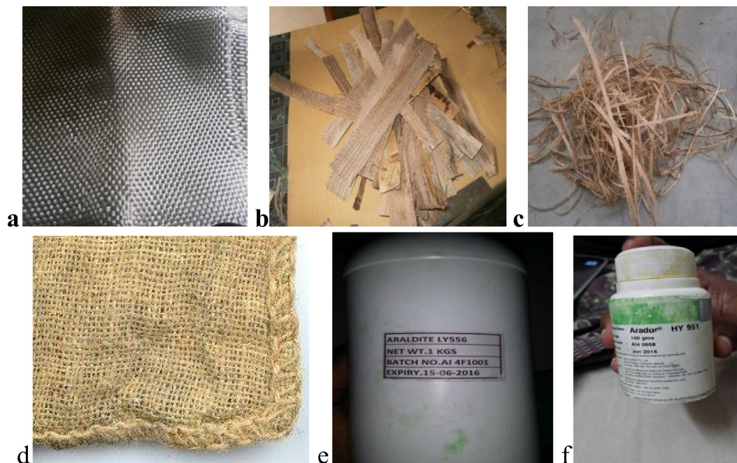
Fig. 1. Hybrid Composite Matrix materials: a) Glass fibre b) Raw banana fibre c) Treated Banana fibres d) Jute fibre e) epoxy f) Hardener.
