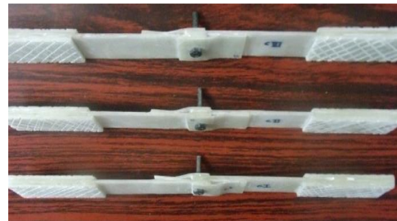
Fig. 3.3. Hybrid joint with curved attachment (24°).
