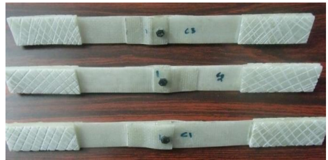
Fig. 3.2. Hybrid joint with curved attachment (12°).
