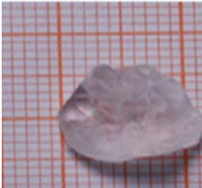
Fig. 1: Grown crystal of L-Histidine doped Potassium Fluoride
