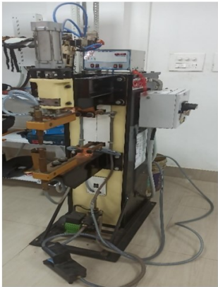
Figure 6.3: Electro-weld (SP50) RSW machine
