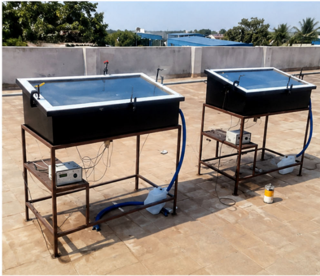
(a) Experimental setup of single-slope still system
