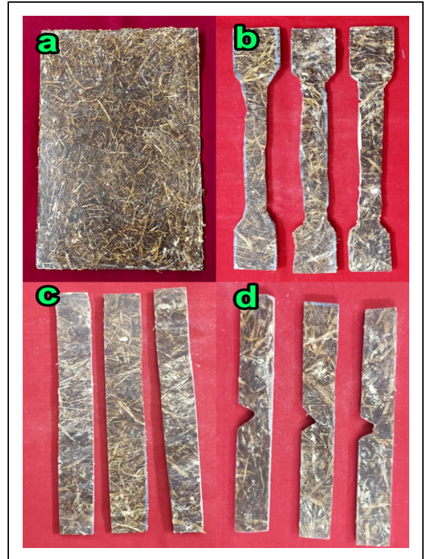
Fig. 2: Images of (a) composite laminate specimens of (b) tensile test, (c) flexural test and (d) impact test
