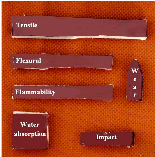
Fig. 4 Photographic view of testing specimens
