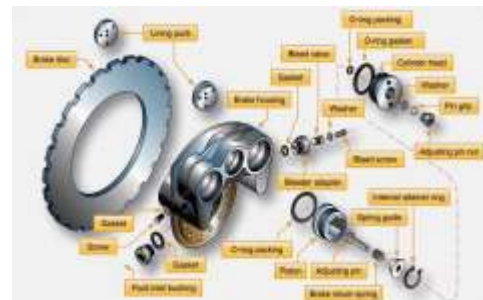
Figure: Exploded view diagram of a single-disk aircraft brake assembly
