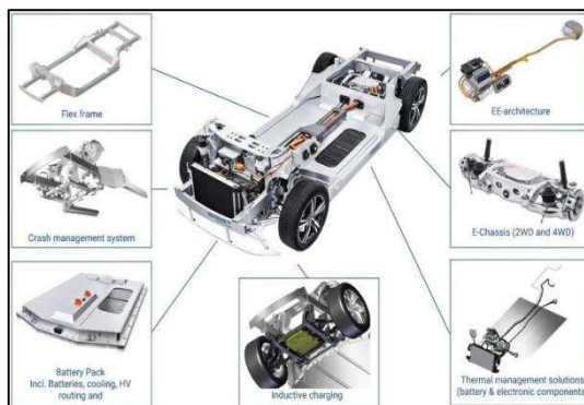
Fig. 5. The 3D model-style illustration of the skateboard platform architecture for an electric vehicle [39]
