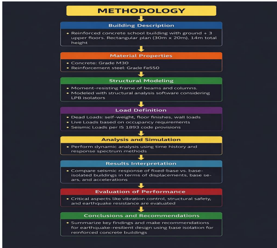
Figure.3: Methodology of reinforced concrete study
