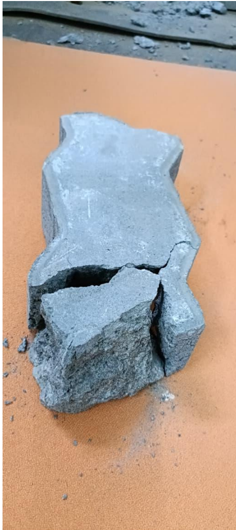
Figure 3: Paver Block (with 12.5% SDA)
