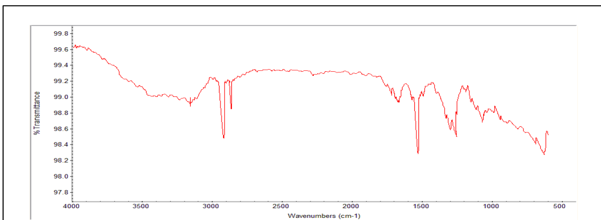
Figure 4 (A). FTIR spectra of PVA
