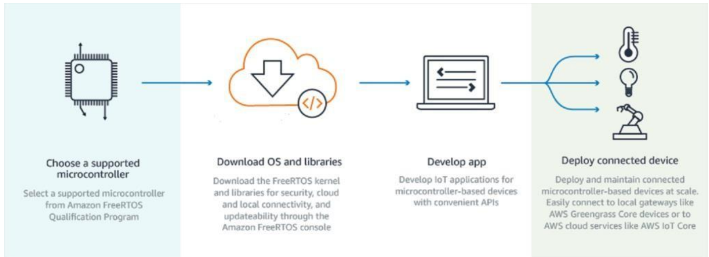
Figure 2: A step-by-step display of how an MCU-based IoT device can be connected to a cloud service like AWS IoT Core. (Image: CNX Software)
