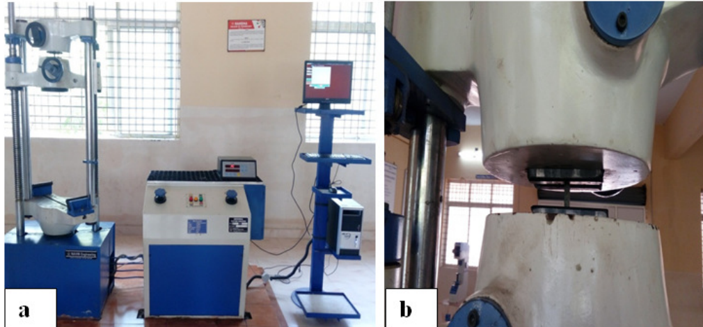
Figure 3 (a) Universal Testing Machine (b) specimen fixed in UTM cross head between flat jaws
