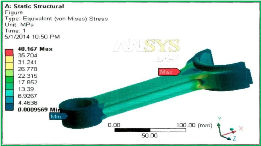
Figure. 5: Von-mises Stress at 'H' section
