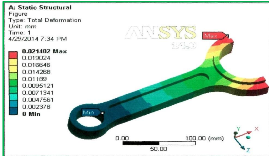
Figure. 2: Total deformation at 'I' section
