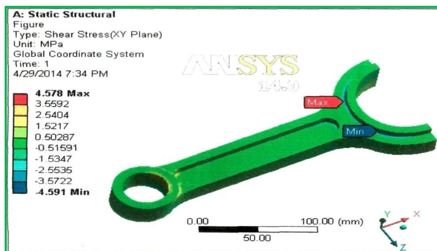
Figure. 4: Shear Stress at 'I' section
