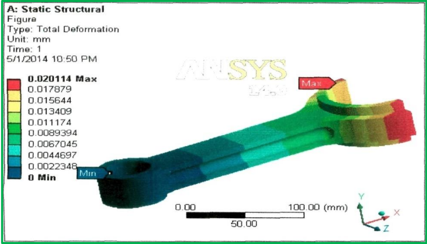
Figure. 6: Total deformation at 'H' section
