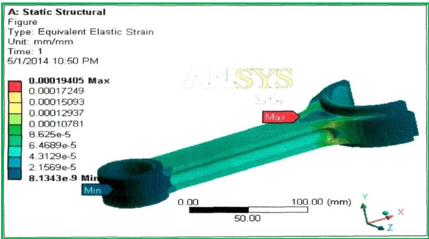
Figure. 7: Elastic Strain at 'H' section
