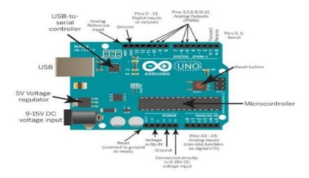
Arduino Uno consists of 14 digital input/output pins (of which 6 can be used as PWM outputs), 6 analog inputs, a 16 MHz crystal oscillator, a USB connection, a power jack, an ICSP header, and a reset button
