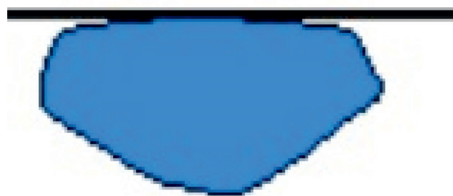
Normal moisture distribution in clay soil
