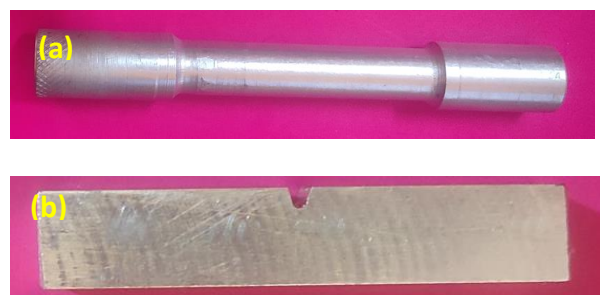
Fig. 3. (a) Tensile test specimen sample of A356-9wt.% of 40 \mu\text{m} \text{B}_4\text{C} composite (b) Impact test specimen sample of A356-9wt.% of 40 \mu\text{m} \text{B}_4\text{C} composite
