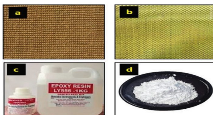
Figure 2. Photographic images of (a) Piassava fiber; (b) K-29 Kevlar fiber; (c) LY556 epoxy matrix with hardener and (d) \text{SiO}_2 NPs
