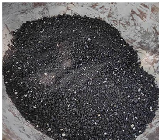
Figure 5: Graded Steel slag confirming to Zone 11 (IRC 15-2017 & IRC 44-2017).
