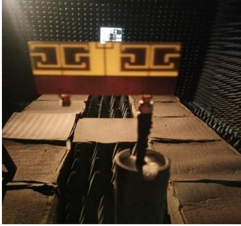
Fig. 9 Antenna connected to VNA machine
